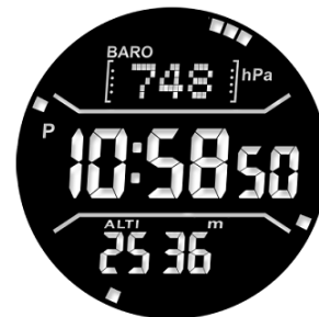
Monochrome display simultaneously displaying time and measurement data (image shows an example of atmospheric pressure/altitude and compass bearing)
